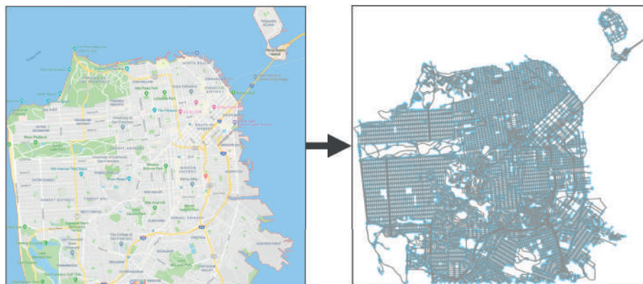
Figure 2. Image of San Francisco – CA, USA, extracted from Google Maps (on the left-hand side) and created using OSMnx (on the right-hand side).
