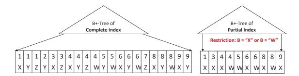
Figure 1. Representation of scanned data entries in Partial and Complete indexes for Query Q: A > 0 and A < 10 and B = X. Values for attribute A are represented in the first row of leaf nodes, while values for attribute B are in the second row.
